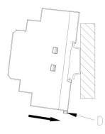
Removal: Insert the screwdriver into E, pull down the snap and make it tilt outward in the meantime, then it can be removed from the rail.
